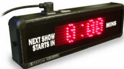
Right: 5 Character static display with reset and controller via PC link. 60mm Ch Ht internal Red LED Display. (Longleat Miniature Railway)
