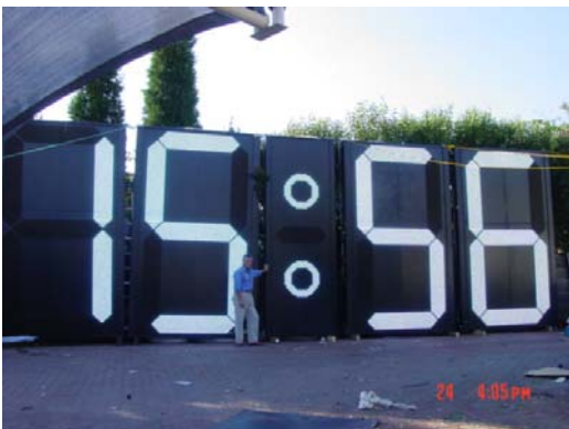
Above: 4metre electromechanical clock controlled by master clock controller
