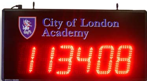
Left: 140mm Ch Ht ultrabright Red LED countdown clock with internal casing spec. (City of London Academy)
