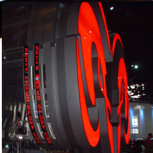
Photos show built in (bespoke) single line displays. Note the orientation of the characters in the red display and the slight curve to the display boards. Blue—100mm ch ht. Red—60mm
