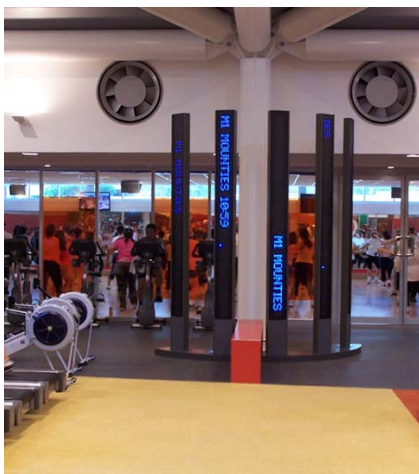
Photos show built in (bespoke) single line displays. Note the orientation of the characters in the red display and the slight curve to the display boards. Blue—100mm ch ht. Red—60mm
