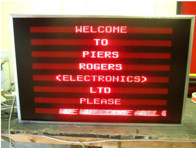
Left: A standard multiline display consisting: 8 line 24 character 30mm red LED's for display of reception information or used to display general auction information.
